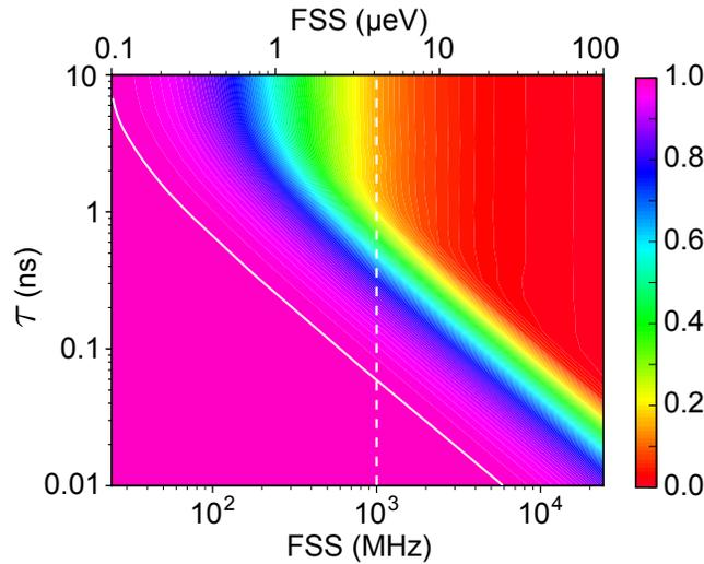
Fig. 2. The measurable entanglement represented as the averaged concurrence  $\bar{C}$  as a function of the detector time resolution ( $\tau$ ) and fine-structure splitting (FSS) in case of an exciton lifetime of  $\tau_X = 1$  ns. The white dashed line is a guide to the eye for the examples in the text and the white solid line highlights the 0.99 contour line.
