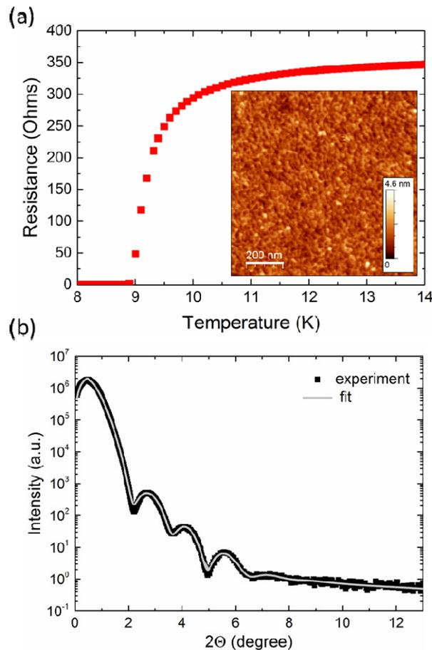
Fig. 1. (a) Film resistance vs. temperature for the NbN thin film under study. Inset:  $1 \times 1 \mu\text{m}^2$  atomic force microscopy image of the NbN surface. (b) X-ray reflectivity of the NbN film on  $\text{SiO}_2$ -on-silicon. Black squares are experimental measurements and the solid gray line is a fit generated with the GenX software.
