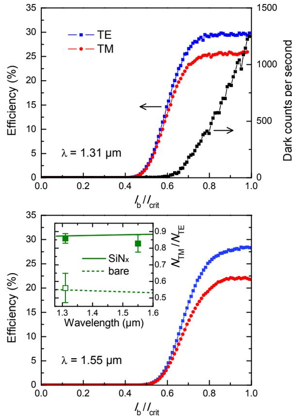
Fig. 5. Detection efficiency as a function of the bias current / critical current ratio ( $I_b/I_{crit}$ ), measured for a typical SNSPD device (a) at 1.31  $\mu\text{m}$ , and (b) at 1.55  $\mu\text{m}$ . The dark count rate is represented in (a). Inset in (b): measurement of the  $N_{TM}/N_{TE}$  response ratio of bare devices (open symbol) and devices capped with  $\text{SiN}_x$  (solid symbols). The curves represent theoretical calculations for both cases.
