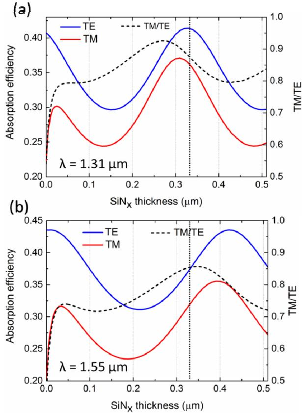
Fig. 4. Calculated dependence of TE and TM absorption efficiency, as well as the TM/TE absorption ratio, as a function of the thickness of the SiN<sub>x</sub> cap layer at (a) 1.31 μm, and (b) 1.55 μm.
