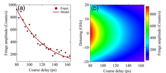
**Fig. 4.** (a) Determination of  $T_2^*$  using the decay of the Ramsey fringe amplitude as a function of the coarse delay. Note that the initial delay that is used in this experiment is 80 ps. The solid red line is a fit from the model with a decay time of 43 ps. (b) Modeled Ramsey fringe amplitude decay as a function of the coarse delay for a range of resonant pulse detunings. Although the amplitude gradually reduces when the detuning is increased, the decay time remains the same.
