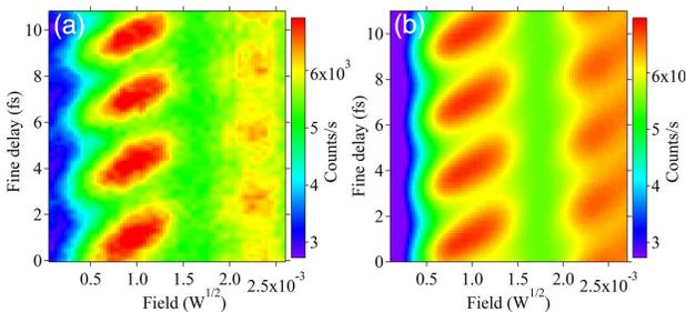
**Fig. 5.** (a) Detected counts when the system is manipulated with two pulses of variable power and variable delay. This allows access to the full Bloch sphere (complete coherent control). The tilt of the lobes for low pulse powers originates from the non-zero detuning of the resonant pulses used in this experiment ( $\Delta\omega_L/2\pi \sim 14.5$  GHz). (b) Modeled complete coherent control, with parameters set to match those used in the experiment.
