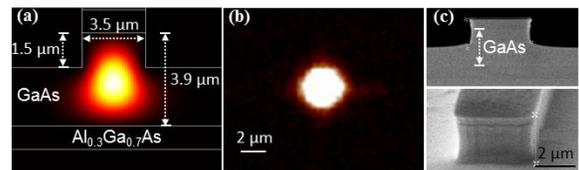
Fig.1. (a) Cross section of the GaAs/Al<sub>0.3</sub>Ga<sub>0.7</sub>As ridge waveguide and its simulated field distribution of the TE fundamental mode at 1550 nm wavelength, (b) measured intensity distribution of the TE fundamental mode at 1550 nm wavelength and (c) Scanning Electron Microscopy (SEM) images of the GaAs/Al<sub>0.3</sub>Ga<sub>0.7</sub>As waveguide.
