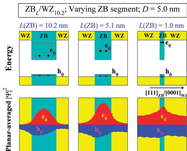
FIGURE 6. Single-particle energy and planar-averaged wave function square for  $e_0$  and  $h_0$  in the  $ZB_L/WZ_{10.2}$  wire with 5 nm diameter. Additional confined states bound in ZB segments are also shown. Note that the  $h_0$  wave function is not symmetrically centered in the ZB section, which might result from the influence of the asymmetric WZ potential as mentioned since the confinement potential well of holes is shallow.
