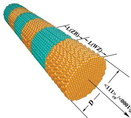
**FIGURE 1.** Schematic structure of the wurtzite/zincblende superlattice nanowire, defined with the wire diameter  $D$  and altering the ZB segment length  $L(\text{ZB})$  and the WZ segment length  $L(\text{WZ})$ .
