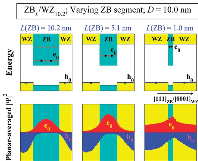
FIGURE 5. Single-particle energy and planar-averaged wave function square for  $e_0$  and  $h_0$  in the  $ZB_L/WZ_{10.2}$  wire with the 10 nm diameter. Here (and following Figure 6) band offsets are based on calculated band edges for pure ZB and WZ wires with the same diameter.
