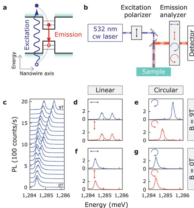
**Figure 2.** Polarization-sensitive magneto-photoluminescence of a single nanowire quantum dot. (a) Schematic of nonresonant excitation and recombination. (b) Experimental setup. The excitation polarization is vertically linearly polarized, whereas the polarization of the emission is analyzed. (c) PL for different magnetic fields in steps of 0.5 T. Emission polarization is not filtered. (d–g) PL with linear and circular polarization filters for 0 and 9 T.
