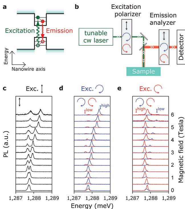
**Figure 3.** Polarization-selective excitation and detection of exciton spin states. (a) Schematic of quasi-resonant excitation and recombination. (b) Experimental setup. Both excitation and detection polarizations are varied. (c–e) PL for different magnetic fields. Excitation is linearly, right circularly, and left circularly polarized, respectively. Emission analyzers are set to linear (black), right (blue), or left (red) circular polarization.
