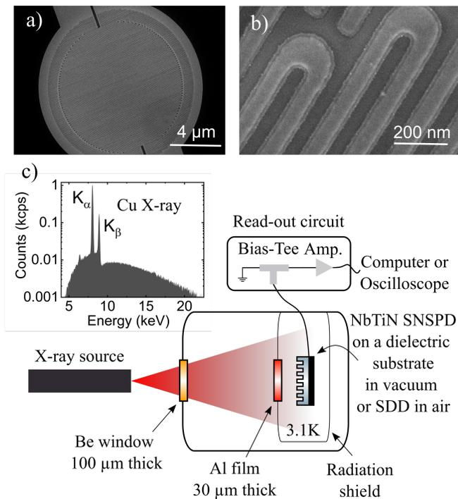
Fig. 1. (a,b) Scanning electron microscope images of the NbTiN detector revealing its structure: circular area with  $10 \mu\text{m}$  diameter, and 0.5 filling factor. (c) A diagram of the experimental setup. A copper X-ray source illuminates the NbTiN superconducting single photon detector (X-SNSPD) that is kept at cryogenic temperature of 3.1 K. The inset shows the corresponding X-ray spectrum.
